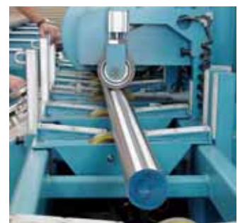
Each shaft is polished to ensure a smooth finish which is critical in the bearing areas and for optimum corrosion resistance.
