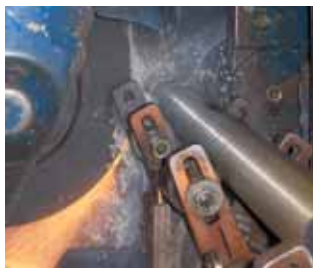
Centerless grinding experts grind the bar to our exacting ring-gage specifications.
